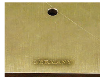
▼ Figure 14-9: German Elite Movement Plate with “GERMANY” Signature From a 1904 Herschede Pattern No. 140 Courtesy of Covenant Clock Restorations, Beaverton, OR
