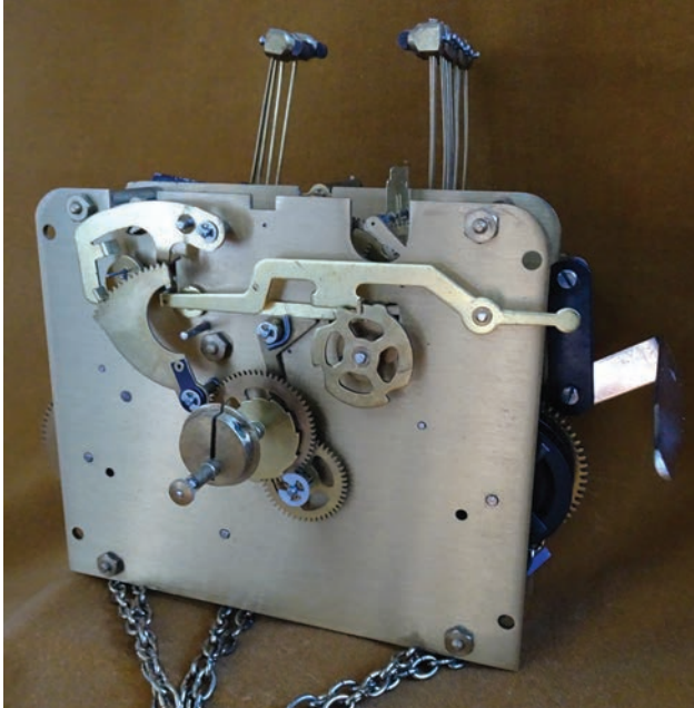
▼ Figure 14-23: Circa 1975 Herschede Chain-Wound Model 1200 Movement Front
